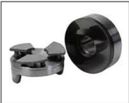
Kingsbury type thrust bearing unit consisting of tilting pads made of highly-resistance stainless steel and machined by tesla using the spherical lapping process.
