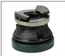
Kingsbury type thrust bearing unit consisting of tilting pads made of highly-resistance stainless steel and machined by tesla using the spherical lapping process.
