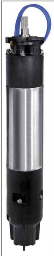
8" asynchronous two-poles or four-poles submersible motor, rewindable-type made in AISI 316 stainless steel and supports in cast iron with paint coating (standard version). Cooling and lubrication of the thrust bearings assembly and carbon bushes is provided by a mixture of water and glycol.
