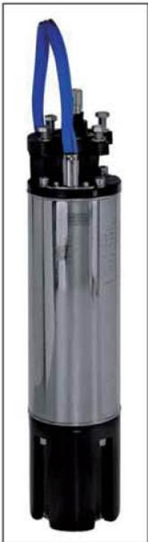
6" asynchronous two-poles submersible motor, made in AISI 304 stainless steel and cast iron with paint coating for parts in contact with water. Cooling and lubrication of the thrust bearings assembly and carbon bushes is provided by a mixture of water and glycol. Squirrel-cage rotor mounted on kingsbury self-centering thrust bearing. Stator housed in an airtight stainless steel casing (canned-type).
