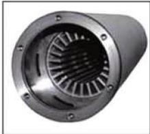
(Stator is rewindable type and its inserted in an AISI 316 stainless steel outer shell in the standard version the windings are made in copper insulated by PVC On request its available the PE2+PA windings for special applications such as the use with a variable frequency drive.
