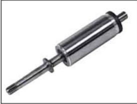
Shafts made of AISI 304/Duplex with a special process of surface hardening and polishing of the working area of the bushes. Squirrel-cage rotor made in aluminium .
